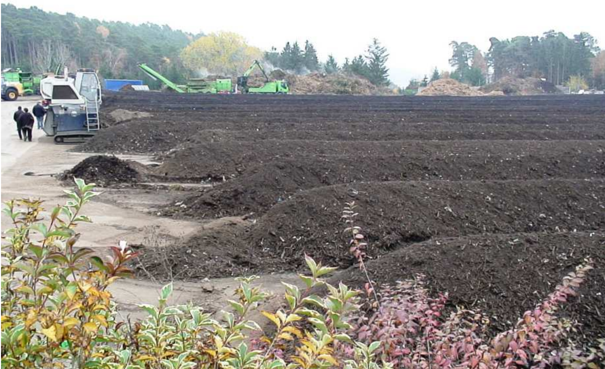
Figure 12: Example of open windrow composting (Binner, 2008)
